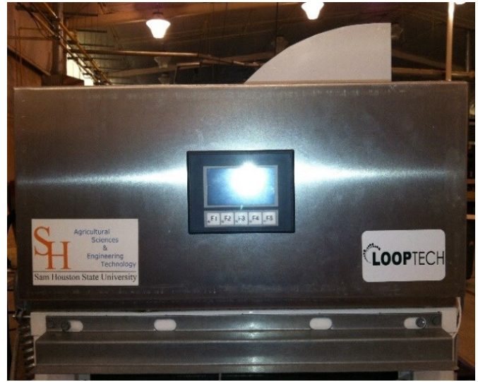
b) PLC Monitoring Display
